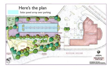
A key feature of the project is an overhead steel structure with 680 solar panels that will generate enough electrical energy to offset 55 percent of the electricity from PG&E that the Patch uses. These panels will provide shade for 48
